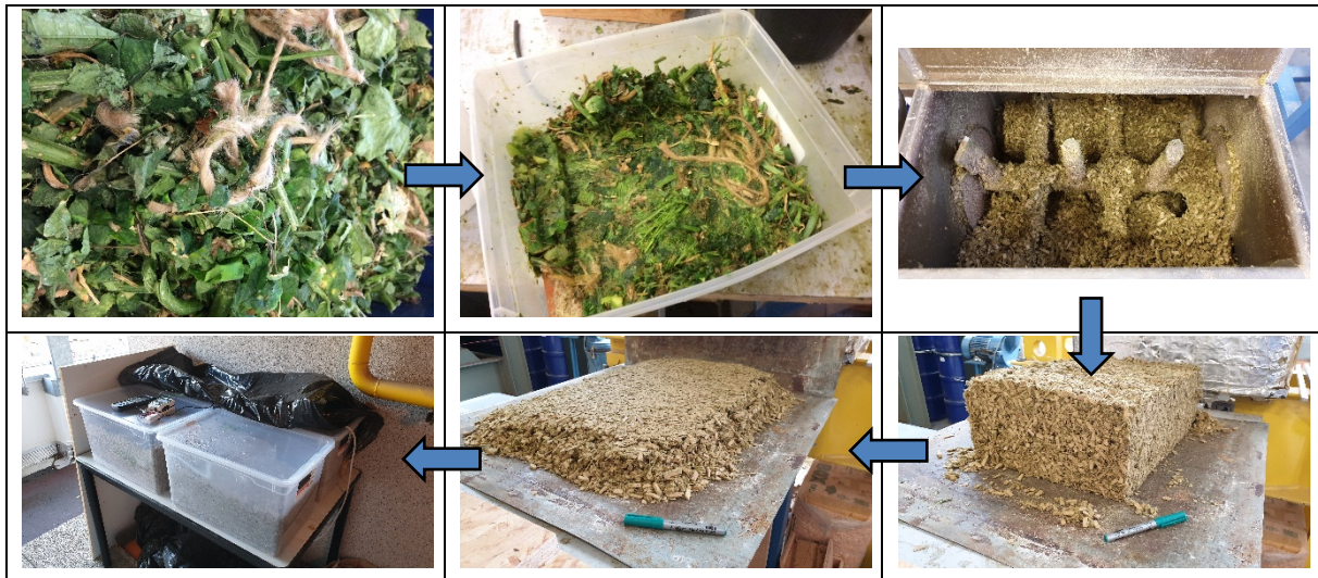
Fig. 2: The main steps of making a “cake” of MDF chips and cucumber waste.
