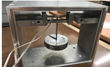
Fig. 3: The 4-point bending setup
