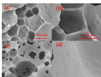
**Figure 3.** The morphological characteristics of tannin-humins foams. (a) and (b) is the foam obtained under 23°C; (c) and (d) is the foam obtained under 80°C
