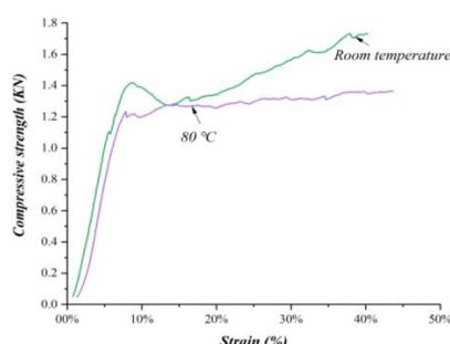
**Figure 4.** The compression curves of tannin-humins foams
