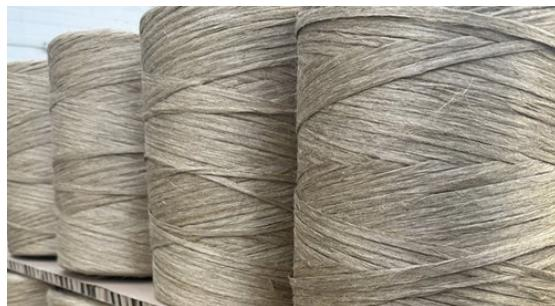
Fig. 1 Flax fiber roving [Depestele]
