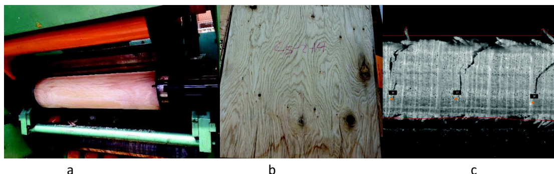
Figure 1. a) Rotary peeling machine, b) Veneer made from secondary quality Oak, c) Measurement of lathe checks depth and frequency using SMOF device
