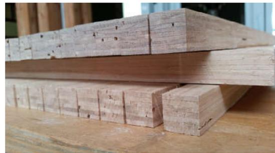
Figure 2: LVL specimen for the measurement of mechanical properties
