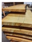
Fig. 9: pith crack on the top end of a twenty-two millimetres board, photo by the author.
