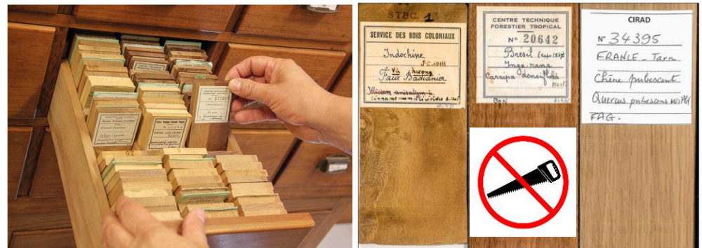
Parallelepiped samples with fixed dimensions ~ 13 cm x 6 cm x 1 cm
