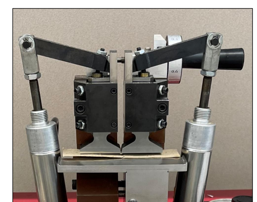
Diagram of a sample, picture of a sample inside the zero-span machine with a zoom on the clamping part
