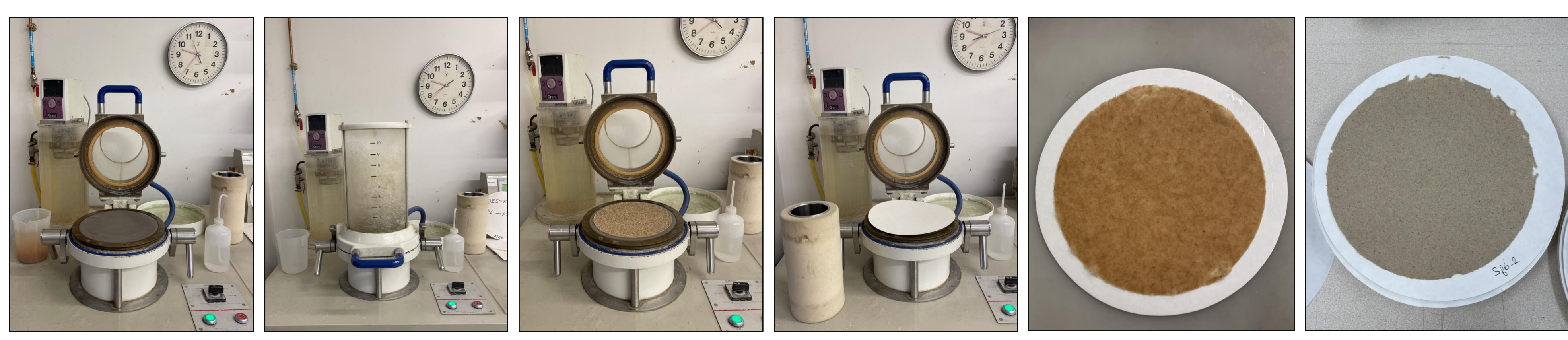
Pictures of different steps of paper making and of the handsheet before and after pressing and heating
