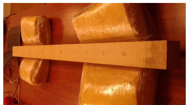
Experiment of adhesive free laminated timber beams with free – free condition
