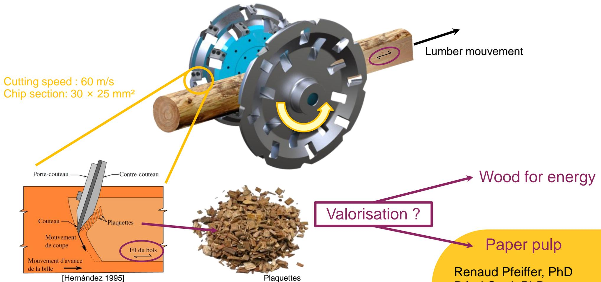
Machined volume ( $\approx 30\%$ ) transformed into chips during the process
