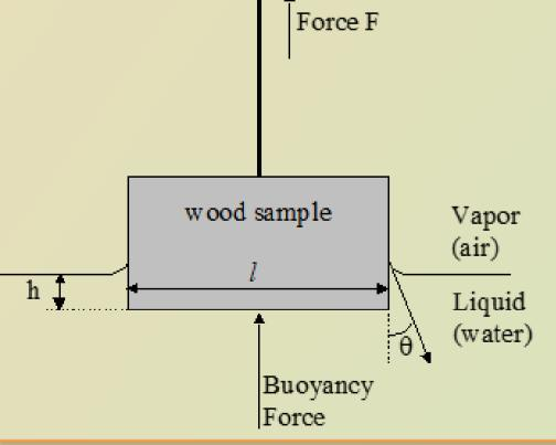
This figure is a schematic diagram of the Wilhelmy method. Immersing a sample plate (width I) of wood into a probe liquid (water) along an immersion depth (h) and pulling it out allows the calculation of advancing and
