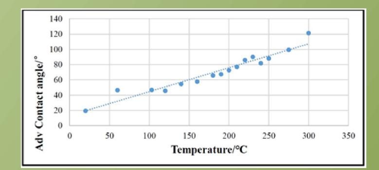
These two graphs are the advancing contact angles of beech and fir heattreated at different temperatures, tested by the Wilhelmy method. All the measurement of the receding contact angle are equal to zero, that means that before and after the treatment the wood cannot be dewetted by the water. It can be seen from the figure that the advancing contact angles of beech and fir both show a trend of increasing first, then flattening, and finally increasing.
