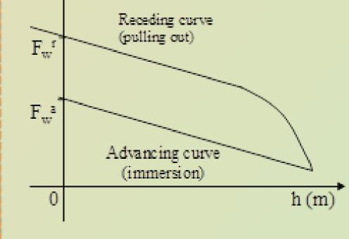
$Fw = cos\theta \gamma P$ Equation 2Where  $\gamma$  is the liquid surface tension andP is the sample perimeter.
