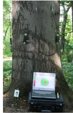
Figure 63 : Tomographe ArborSonic 3D ( http://www.fakopp.com/ ).
