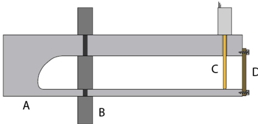
Fig. 1 : Schematic cut of the “Fork” apparatus composed of an aluminum fork (A), a movable blocking member (B), an LVDT (C) and a sample (D) screwed to the free end of the fork.
