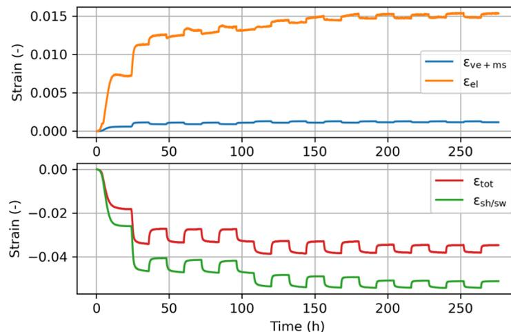
Fig. 3 : Evolution of the different contributions to the total strain measured on the sample placed in the fork device.
